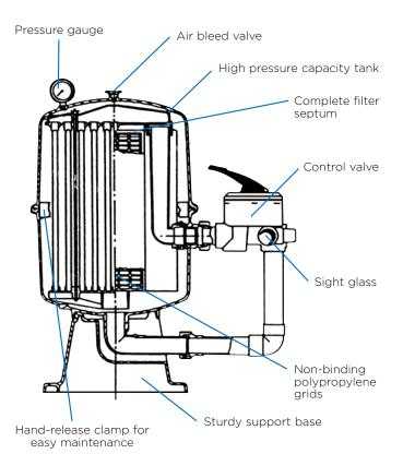
Built to endure the rigours and pressures of the outdoor environment, Fulflo DE filter housings are made from specially engineered polymers that have been tested for durability and strength.
