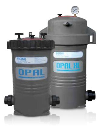
Opal cartridge filters are designed to house an extra large filter cartridge, maximising its dirt holding capacity and minimising filter maintenance. The filter's ergonomic lid allows easy access to the filter cartridge for removal, cleaning and installation in a matter of minutes.
