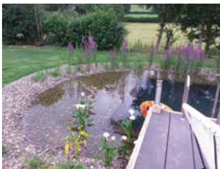
The natural pool's regeneration area where impurities are absorbed by plants as nutrients and harmful bacteria are destroyed by natural water organisms.
