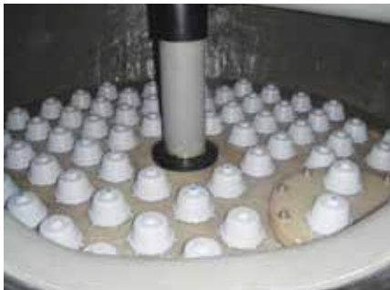
Micron SPDD filters incorporate a patented nozzle plate system which promotes uniform water flow when filtering and backwashing.
