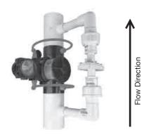
Figure 1.3 Dynamic Venturi Injector (DVI).
